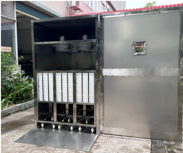
Customized Noodle dryer with customized trolley and air duct.
