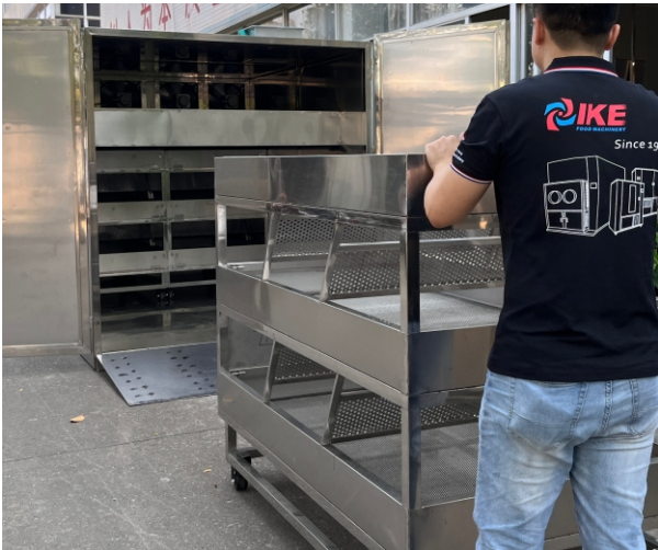
Customized loading basket for stackable products.
