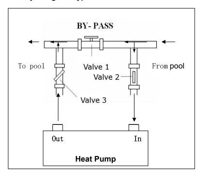
Use the following procedure to adjust the bypass:
