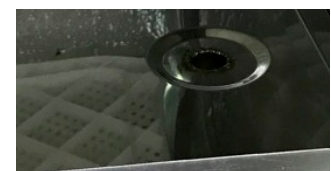
Water outlet for water collection tray
