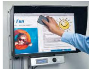
Above: iQ sensor (shown in use with LCD mounted on EVS-2540/iQ) calibrates light level of the viewing station to match the monitor
