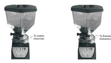
The disk remains in the chosen position without having to be locked in place. The adjustment must be performed with the motor on, and preferably without any coffee between the grinding blades. Grind small amounts of coffee in order to determine the optimal degree of fineness.
