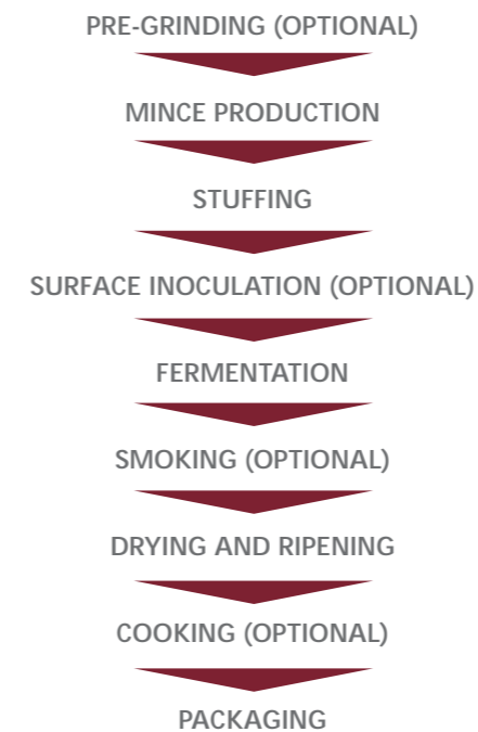
Figure 1. General flow diagram of sausage production
